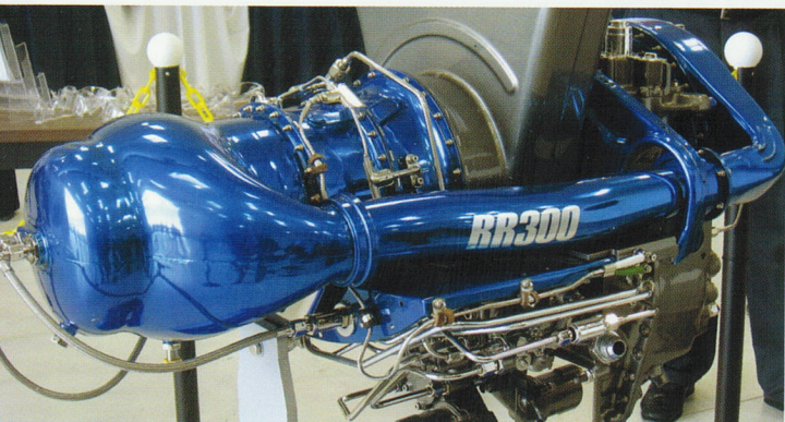
The under-development Robinson R66 was the star of a reception for customers and the press at Robinson's factory in Torrance, California, during Heli-Expo 2009. Next to the turbine-powered helicopter on prominent display was the newly certified Rolls-Royce RR300 turboshaft engine, developed specifically for the R66.
